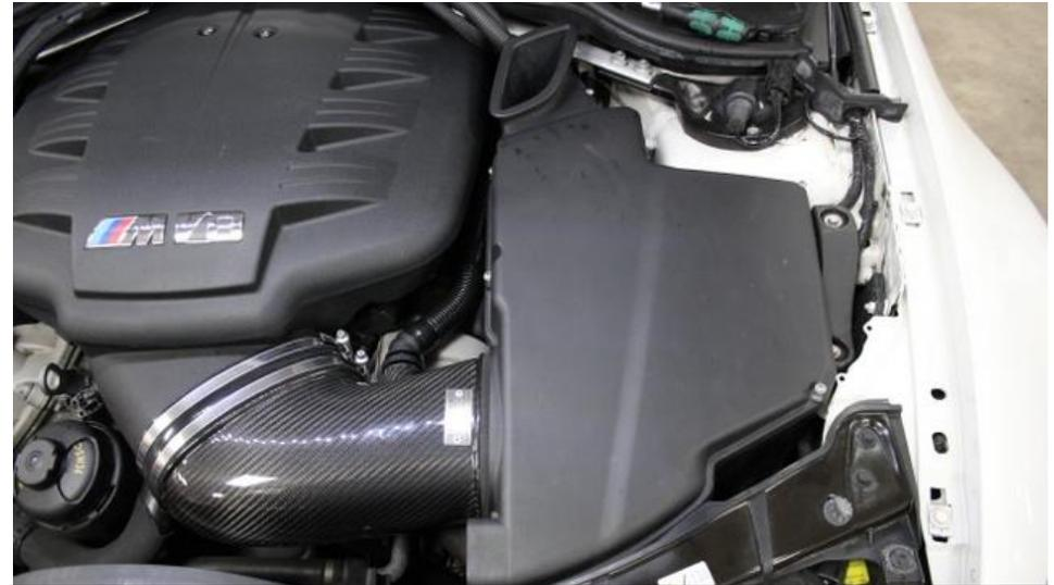
14. Put the airbox lid back on and tighten the Torx screws.
