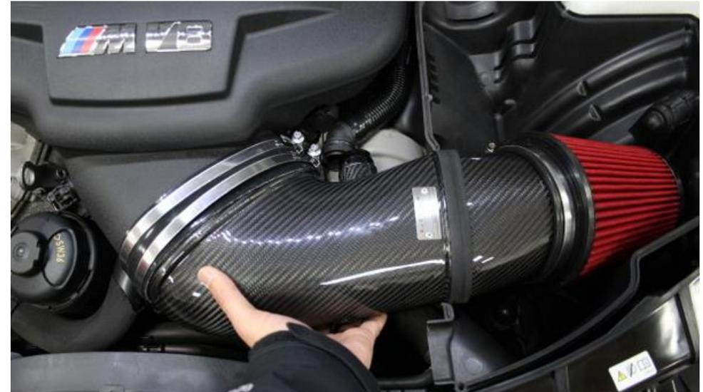
8. Lower the tube into the box and push into the silicon hose – ensure the clamp around the silicon is loose.
