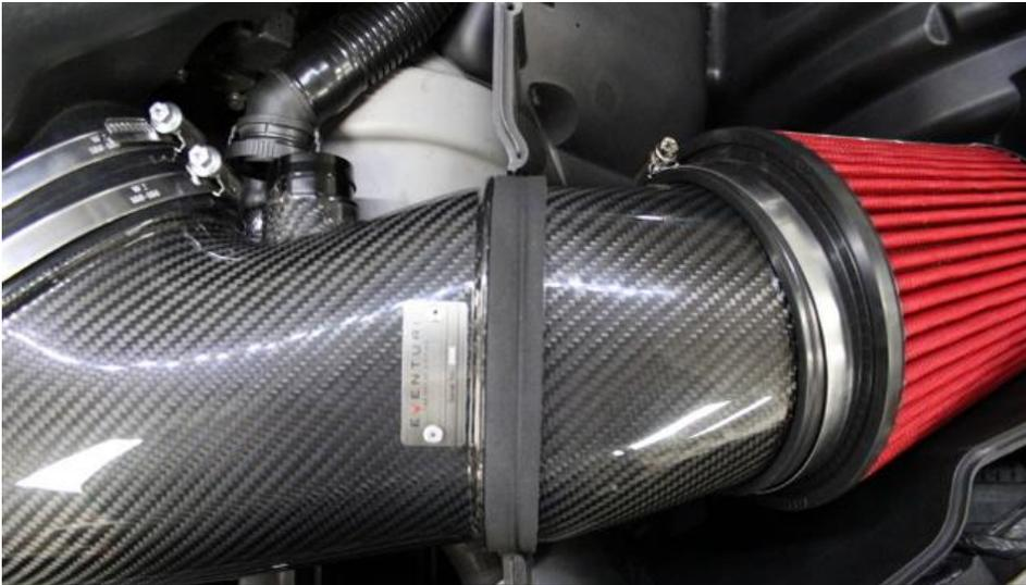
13. Now tighten the clamp around the filter – you can use an 8mm socket to ensure it is tightened.
