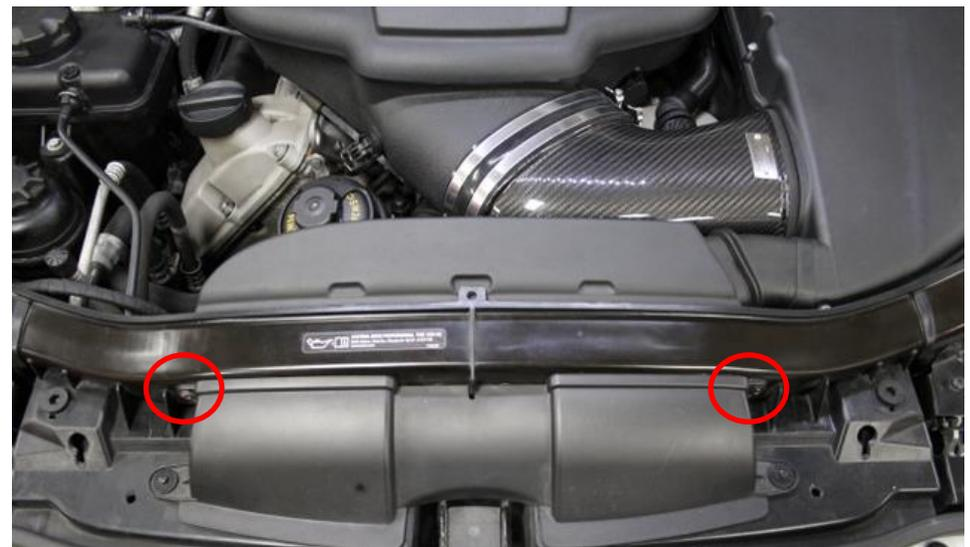
16. Insert and tighten the screws for the duct again.
