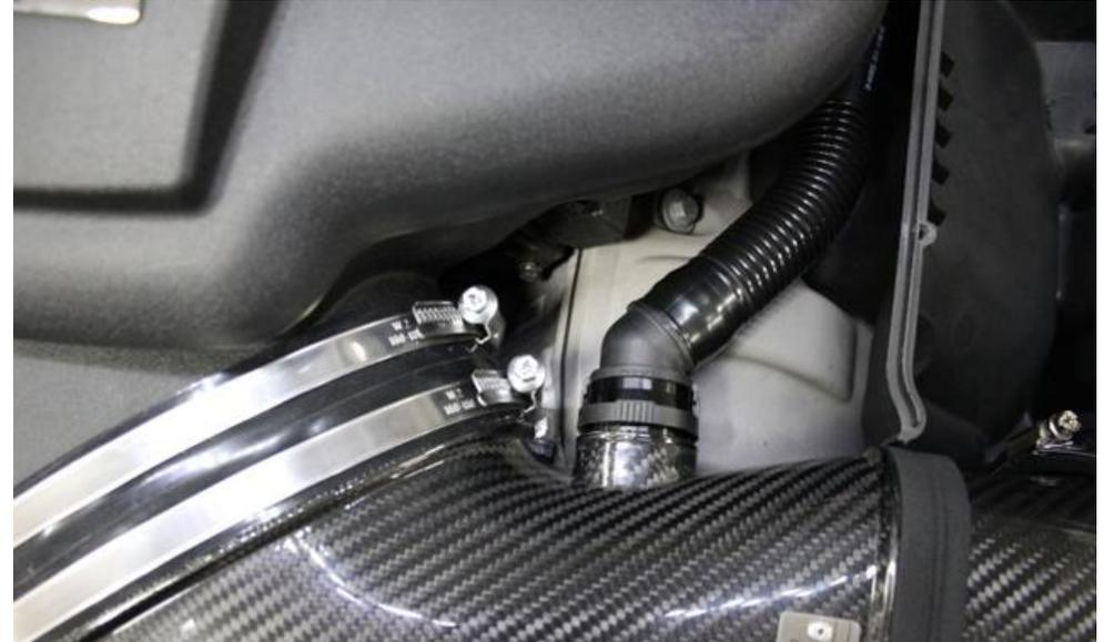
10. Tighten the remaining hose clamp and also insert the breather tube into position. It will click into place.
