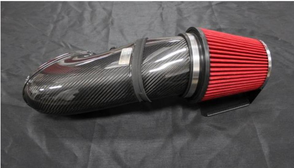
7. Push the filter onto the carbon tube and rotate the filter so that the debris shield is facing down as shown. Do not tighten the clamp around the filter yet.
