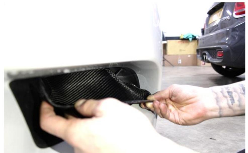
20. Insert the scoop as shown – go underneath the temperature sensor to avoid it. Push the scoop all the way back.
