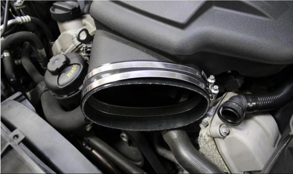
5. Push the silicon hose onto the inlet manifold – make sure it is evenly inserted all around. Place the 2 supplied hose clamps onto the silicon. The clamps are circular but will bend into shape once tightened. See next step before tightening.
