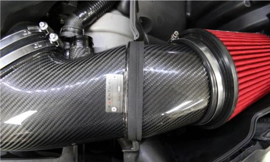
9. Once fully pushed into the silicon it should sit like this with the neoprene band located approximately half way into the airbox.
