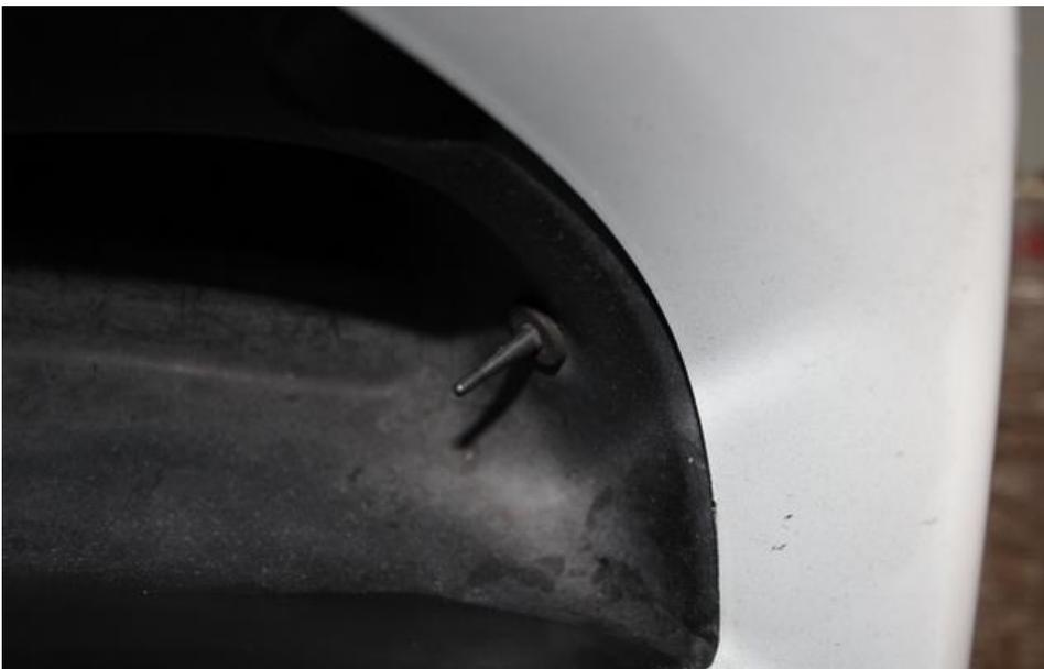
19. Notice the temperature sensor in the duct – you need to install the scoop underneath this.
