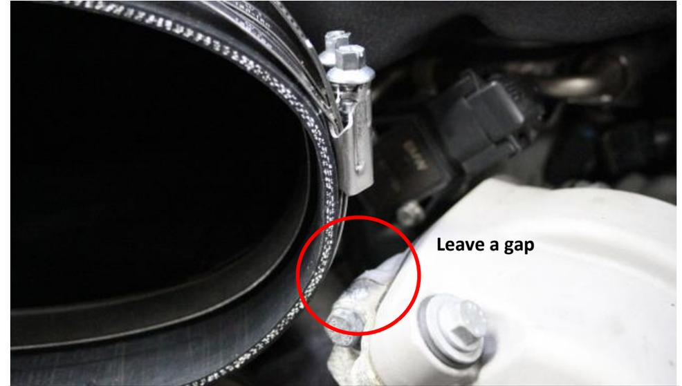
6. Ensure the screw parts of the clamps are away from the circled part of the cam cover. You can also place these screw parts underneath the manifold so that they are hidden. You can now tighten the clamp around the manifold part of the silicon.
