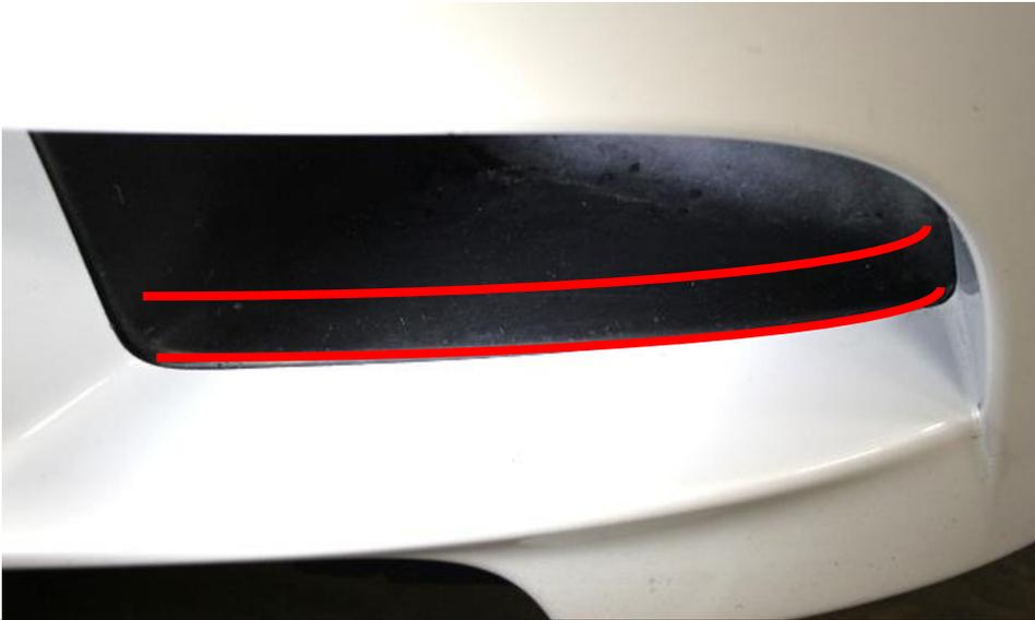
17. Use the supplied 3M wipe to clean the front portion of the intake duct under the headlamp. You only need to clean the first 25mm or so – as shown.
