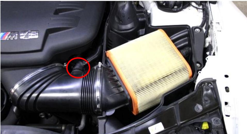
3. Remove the lid from the airbox and you will be left with the stock filter and tube. Loosen the hose clamp around the tube at the inlet manifold. Unclip the breather from the tube as circled.
