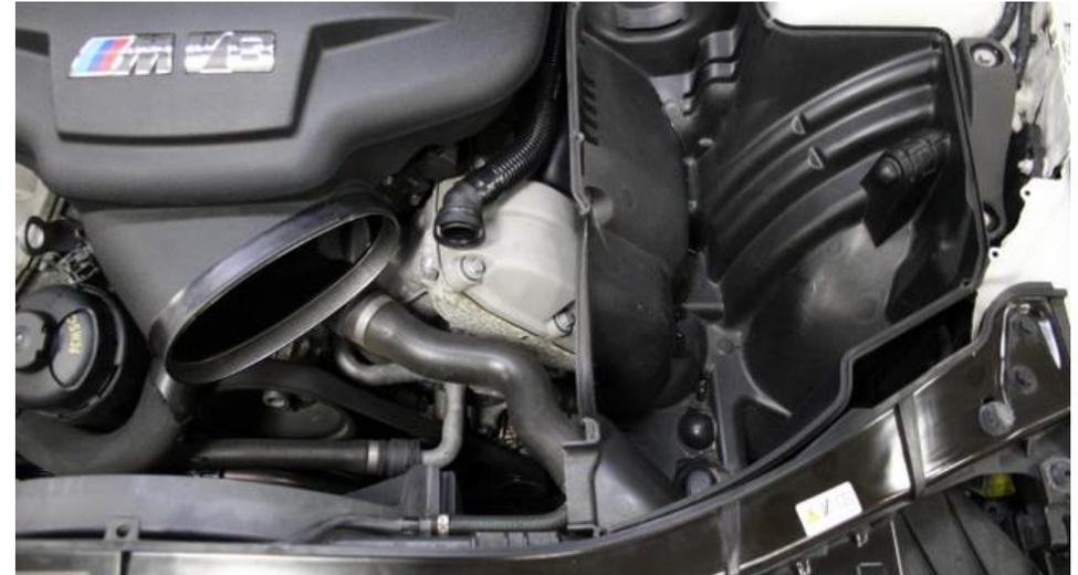
4. Remove the inlet tube and filter from the airbox.
